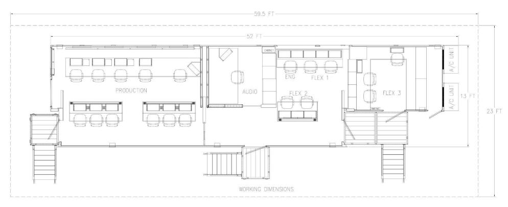
10 Working Positions 60' x 23' Recommended Working Area Single Phase, 208V, 150 Amps
